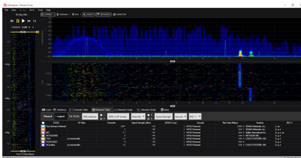
The image above shows MetaGeek Chanalyzer at work scanning a location for a new Wi-Fi install. The only interference we see is above the Wi-Fi spectrum.
