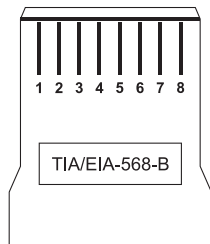
Figure 4. EIA/TIA 568B Termination Pattern
